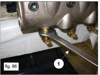
Disassemble the suction and delivery valve units by screwing on an M10 screw long enough to act on the valve and extract the valve guide from the valve seat (1, fig. 87).
